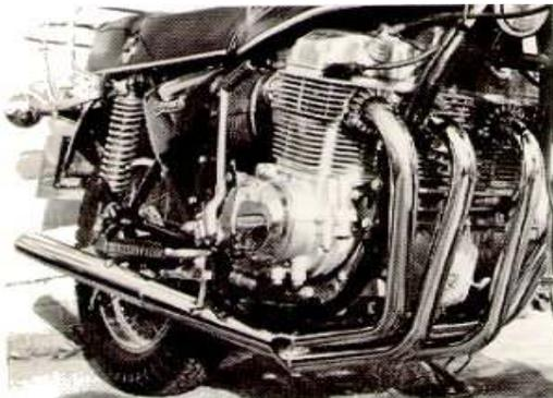
64 *4-into-1 exhaust system on 4-stroke motorcycle.*
