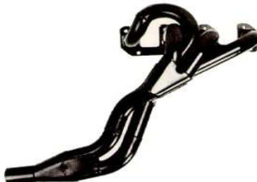
65 *4-into-2-into-1 tuned 4-stroke exhaust manifold.*
